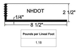
TPER Waterstop is manufactured from a specially formulated Thermoplastic Vulcanizate Rubber. This product has excellent physical properties and chemical resistance and will assure an owner of a facility that require containment for environmentally sensitive materials
