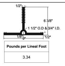
TPER Waterstop is manufactured from a specially formulated Thermoplastic Vulcanizate Rubber. This product has excellent physical properties and chemical resistance and will assure an owner of a facility that require containment for environmentally sensitive materials
