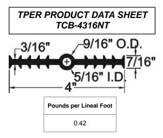
TPER Waterstop is manufactured from a specially formulated Thermoplastic Vulcanizate Rubber. This product has excellent physical properties and chemical resistance and will assure an owner of a facility that require containment for environmentally sensitive materials.
