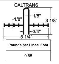
TPER Waterstop is manufactured from a specially formulated Thermoplastic Vulcanizate Rubber. This product has excellent physical properties and chemical resistance and will assure an owner of a facility that require containment for environmentally sensitive materials
