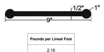
TPER Waterstop is manufactured from a specially formulated Thermoplastic Vulcanizate Rubber. This product has excellent physical properties and chemical resistance and will assure an owner of a facility that require containment for environmentally sensitive materials.
