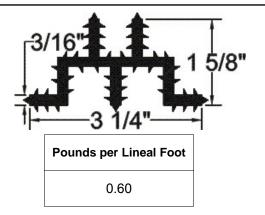
TPER Waterstop is manufactured from a specially formulated Thermoplastic Vulcanizate Rubber. This product has excellent physical properties and chemical resistance and will assure an owner of a facility that require containment for environmentally sensitive materials.
