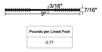
TPER Waterstop is manufactured from a specially formulated Thermoplastic Vulcanizate Rubber. This product has excellent physical properties and chemical resistance and will assure an owner of a facility that require containment for environmentally sensitive materials.
