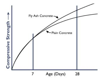
conventional concrete, enabling equivalence at the desired age. This higher rate of strength gain continues over time, enabling fly ash concrete to produce significantly higher ultimate strength than can be achieved with conventional concrete.
