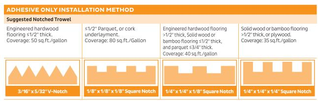
Trowel size is suggested to maximize coverage of adhesive. Periodically check coverage of adhesive during installation: >80% coverage and transfer to the back of the flooring is required for all engineered wood flooring; >95% coverage and transfer is required for all solid wood flooring or bamboo flooring products.
