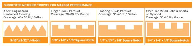
Trowel size is suggested to maximize coverage of adhesive. Periodically check coverage of adhesive during installation; >95% coverage is required for all flooring. Uneven subflooring may require the use of either a leveling/patching material, or a larger notched trowel for proper coverage of adhesive.
