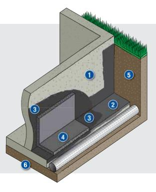
For difficult-to-waterproof below grade substrates, Barricoat-S is the solution. Barricoat-S consists of a water-based modified asphalt emulsion, which is catalyzed to form a seamless, monolithic waterproofing membrane. Perfect for large jobs, Barricoat-S utilizes a convenient spray delivery system that provides a fast application with high mobility which improves overall jobsite efficiency. Barricoat-S can also be applied to green concrete and damp surfaces, which reduces jobsite down time.
