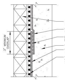
LAGGING OR SOIL RETENTION SYSTEM CCW-MIRAPLY-V WITH BUTYL SIDE FACING OUT HP-250 PRIMER OR LOW-VOC EPDM PRIMER CONCRETE WALL CCW-MIRAPLY-V WITH BUTYL SIDE FACING OUT CCW MIRADRAIN DRAINAGE COMPOSITE WITH FABRIC SIDE FACING LAGGING
