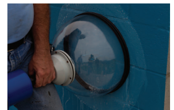
Coating A – Brick Tie Condition No Air Leakage
