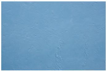
The 60 mil wet coating dries and completely covers the rough substrate.
