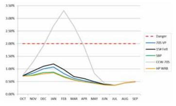
With a missing interior vapor retarder, the wall assembly built with CCW-705 shows unacceptably high moisture levels in the exterior gypsum sheathing. The good thing is that it dries out, due to the permeability of the kraft paper facer. Fire Resist 705 VP and the other permeable WRB products maintain the moisture level of the exterior gypsum sheathing well below the 2% danger level, even when the interior vapor retarder is imperfect or missing.
