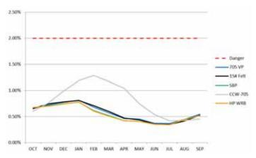
The simulation of the subject wall assembly using each of the WRB products indicates the exterior gypsum sheathing moisture content remains well below the 2% danger threshold. The wall assembly modeled with Fire Resist 705 VP very closely follows the behavior of the other permeable WRB products.
