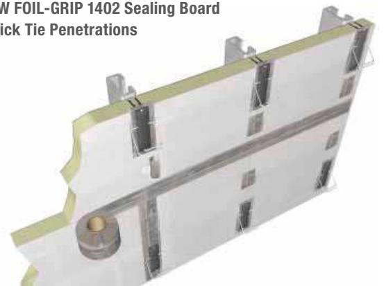
FIGURE 2: Example of Foil-GRIP 1402 Tape Used to Seal R2+ SHEATHE Joints and Penetrations
