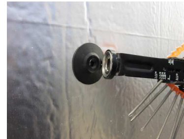
2. Grip-Lok® w/ “Bullseye” adaptor auto-centers over the ci washer
