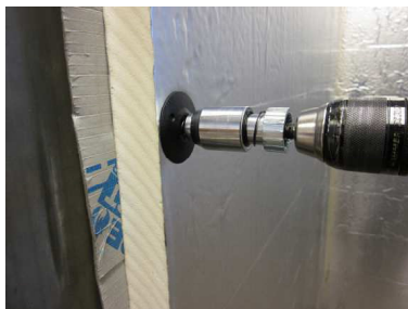
3. EZ-Driver holds screw straight for rapid drilling of steel or wood
