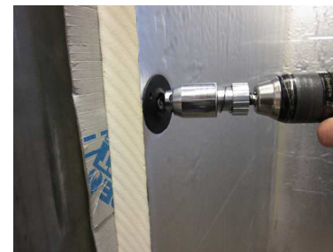
4. EZ-Driver releases fastener at preset depth preventing overdrive
