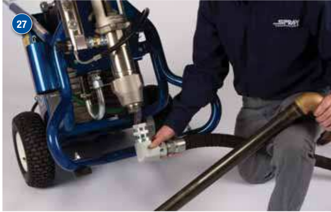
27 Disconnect drum siphon assembly.
