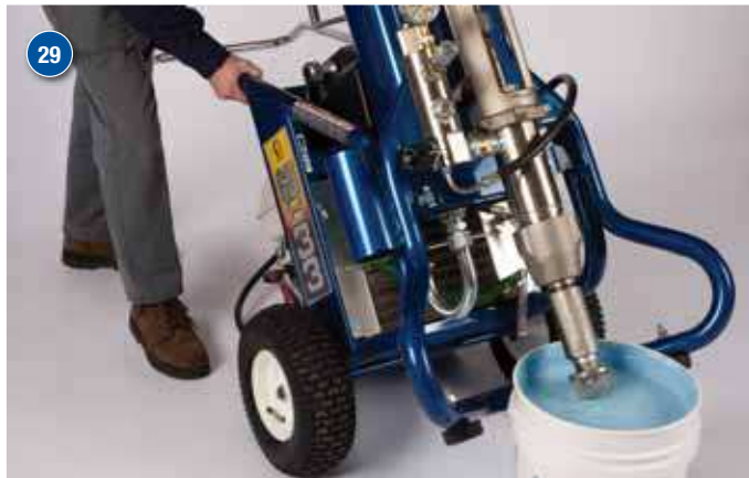
29 Insert siphon end of pump into pail.
