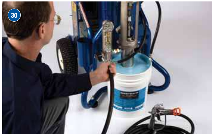
30 Insert purge line into pail. Connect hose and Graco Silver Gun to discharge of Graco pump.
