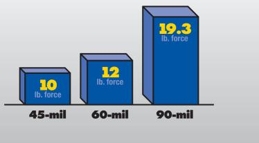
Tested according to ASTM D120
