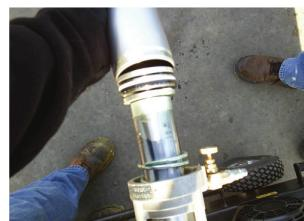
Re-install cylinder taking care to not “cross thread.”
