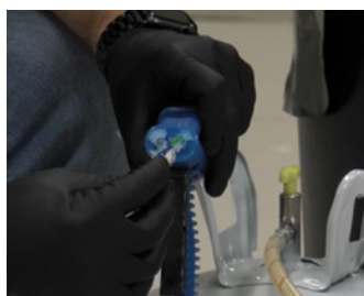
Application of petroleum jelly to spray gun
