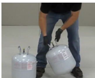
Shaking of A-side and B-side tanks
