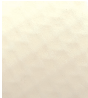
Carlisle's Sure-Weld TPO – 60 Weeks (No Failure)
