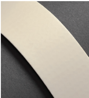
Carlisle's Sure-Weld TPO – 60 Weeks (No Failure)
