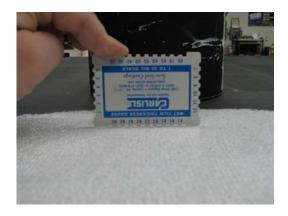
Using the provided wet film thickness gauge, periodically check to ensure proper wet film thickness coverage of the X-tenda Coat Coating (minimum one measurement per square). The wet film thickness gauge should be gently inserted into the applied wet coating making sure that the gauge is perpendicular to the surface area. If the desired wet film thickness is not obtained, additional coating should be immediately applied to the affected areas.
