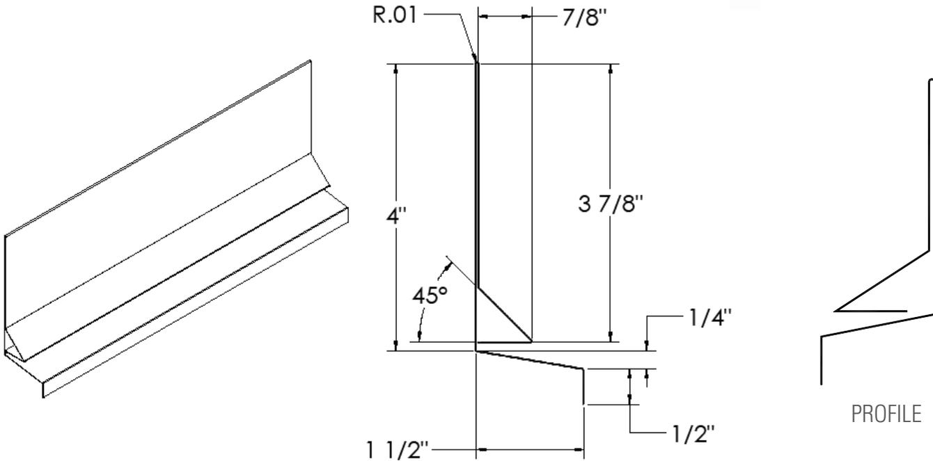
The **#3 FLASHING SCREED** is manufactured for applications above windows, doors and vents on exterior plaster walls. The #3 Flashing Screed consists of a combined single piece 45° weep screed, for drainage, and a Z flashing for window head protection.
