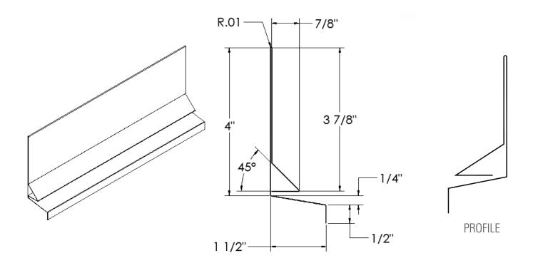
The **#3 FLASHING SCREED** is manufactured for applications above windows, doors and vents on exterior plaster walls. The **#3** Flashing Screed consists of a combined single piece 45° weep screed, for drainage, an a Z flashing for window head protection.
