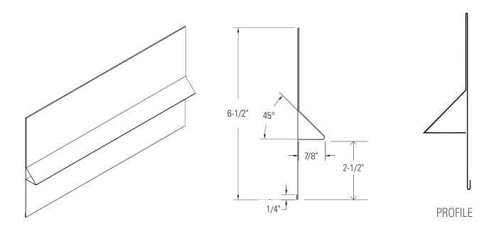
The **#7 EXTENDED FOUNDATION SCREED** provides an additional layer of 25 ga. G90 metal to protect waterproof deck membranes at the base wall from U.V. degradation. The **#7** EXTENDED FOUNDATION SCREED is part of CEMCO's Water Management Products of Stucco Accessories fabricated from minimum 0.018-inch thick hot-dipped galvanized steel complying with ASTM A653 having a minimum G-90 coating complying with ASTM A925. **Water tested per ASTM E1105.**
