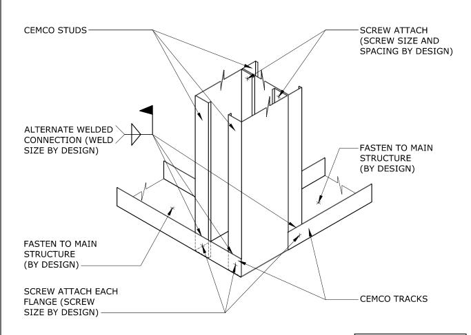
NOTE: STUD MUST BE SEATED TIGHT TO TRACK WEB (MAX. GAP = 1/16")
