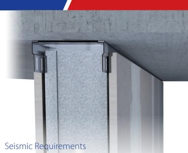
FAS Track 1000 is approved for Class III cycling requirements, 500 cycles at 30 cycles per minute, meeting seismic building codes requirements. The Class III movement provides design advantages over mastic reliant systems which are typically limited to Class II (wind sway) capabilities of 500 cycles at 10 cycles per minute.
