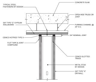
\*NOTE: DOUBLE LAYERS OF 5/8" DRYWALL FOR 2 HOUR FIRE RATING
