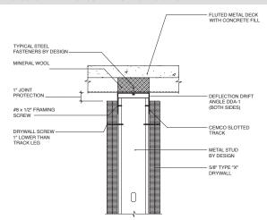
\*NOTE: SINGLE LAYER OF 5/8"TYPE "X" DRYWALL FOR 1 HOUR FIRE RATING, 2 LAYERS FOR 2 HOUR PROPERTY OF 1/8 Property of
