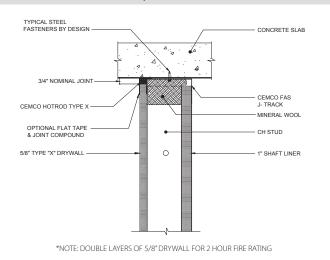
DEFLECTION JOINTS OF 1/2" OR LESS DO NOT REQUIRE ANY ADDITIONAL FLAT TAPE & JOINT COMPOUND.
