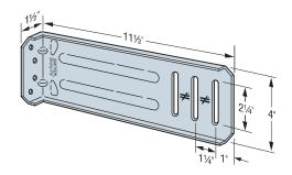
The SCB/MSCB slide-clip connectors are high-performance connectors for bypass framing applications designed to reduce design time and overall installed cost. Various anchorage methods have been tested, and the resulting allowable loads eliminate the need to design connector anchorage. The SCB/MSCB can accommodate applications that typically require two parts with a single connector, reducing material and labor cost.
