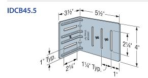
The IDCB drift-clip connector is used to secure bypass stud framing to the edge of a slab. The connector will accommodate 1" of lateral drift in each direction and 1" of upward and downward vertical deflection. Tested load values are provided for anchorage to a steel edge angle using #12 x 1 1/4" Strong-Drive® XL Large-Head Metal screws.
