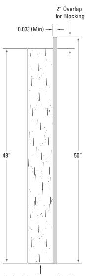
**Typical Fiber Cement Sheathing** (3/4" Thickness)
