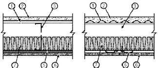
1. Steel Deck — Min 9/16 in. deep, 22 MSG galv corrugated fluted steel deck. Attached to each joist with #10 3/4 in. long screws at each side joint and no more than 12 in. OC between sides
