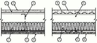
1. Steel Deck — Min 9/16 in. deep, 22 MSG galv corrugated fluted steel deck. Attached to each joist with #10 3/4 in. long screws at each side joint and no more than 12 in. OC between sides.
