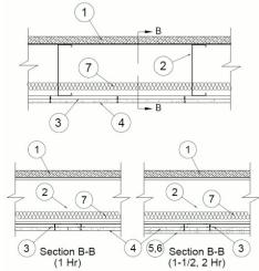
Units, Partition Panel\* — For 1 - 2 Hr Rating - Steel faced panels. Panels secured to top chord of steel joists with #8, 1-5/8 in. cement board Grabber screws spaced 6 in. OC CALIFORNIA EXPANDED METAL PRODUCTS CO - Sure-Board
