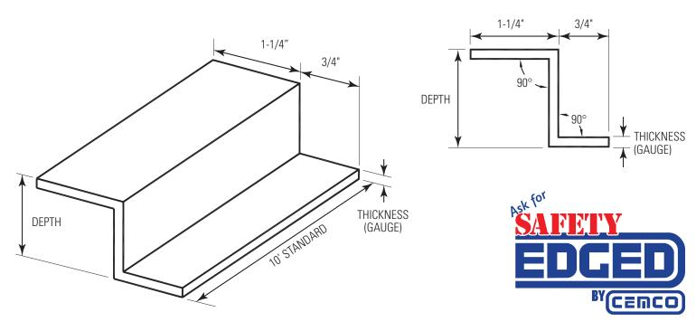
**CEMCO Z-Furring Channel** is fabricated from hot-dipped galvanized steel complying with ASTM A653 with a minimum G40 coating meeting ASTM A924. The furring channel is fabricated from minimum 25 gauge (0.0179" thick) steel (uncoated). The channel is manufactured in various web depths and leg lengths (attachable flange). G60 and G90 coatings are available through special order, and may require up-charges and extended lead times.
