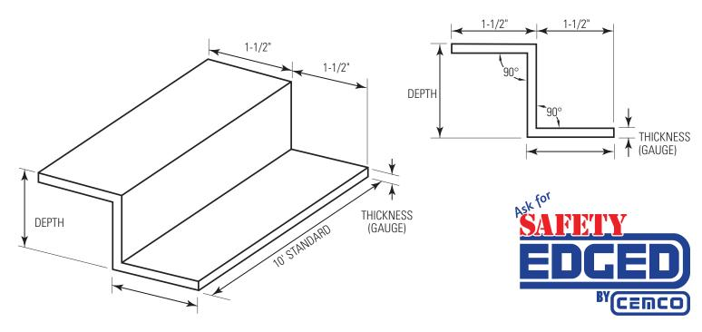
**CEMCO Z-Furring Channel** is fabricated from hot-dipped galvanized steel complying with ASTM A653 with a minimum G40 coating meeting ASTM A924. The furring channel is fabricated from minimum 16 gauge (0.0538" thick) steel (uncoated). The channel is manufactured in various web depths and leg lengths (attachable flange). G60 and G90 coatings are available through special order, and may require up-charges and extended lead times.
