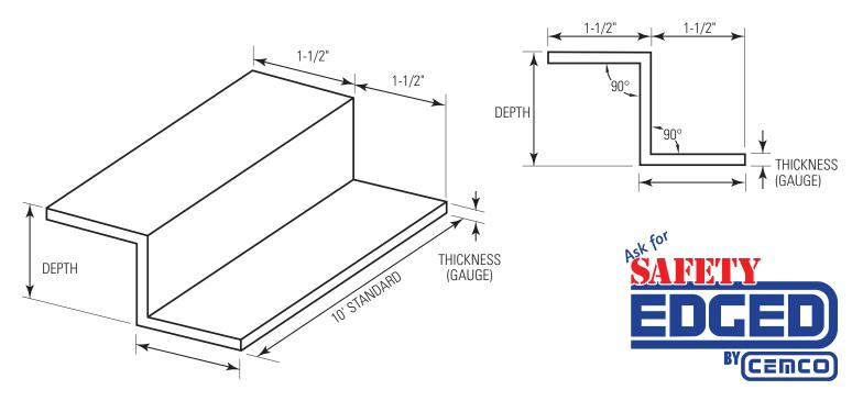
**CEMCO Z-Furring Channel** is fabricated from hot-dipped galvanized steel complying with ASTM A653 with a minimum G40 coating meeting ASTM A924. The furring channel is fabricated from minimum 20 gauge (0.0296" thick) steel (uncoated). The channel is manufactured in various web depths and leg lengths (attachable flange). G60 and G90 coatings are available through special order, and may require up-charges and extended lead times.
