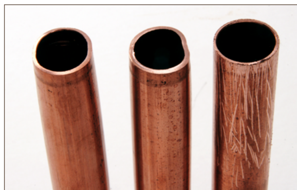
Figure 10.1. Inspect tube for imperfections
