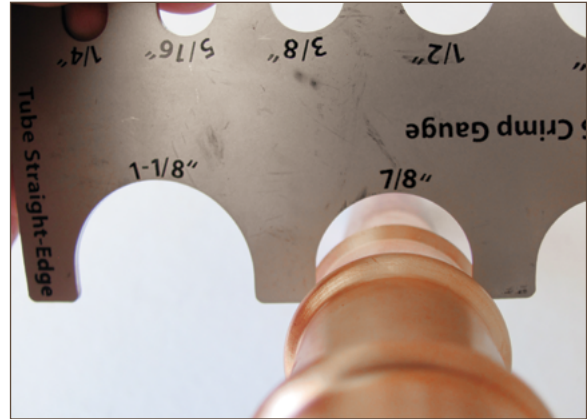
Figure 11.21. Un-crimped or improperly crimped fitting
