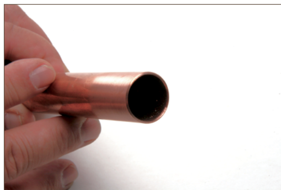
Figure 13.8. Reamed and deburred branch tube end
