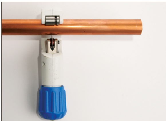
Figure 11.6. Cutting the tube square
