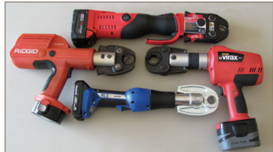
Figure 11.2. Press tools and jaws
