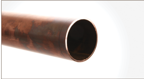
Figure 10.3. Square-cut tube end
