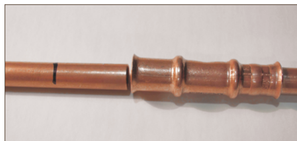
Figure 11.18. Tube marked for insertion into HVACR fitting
