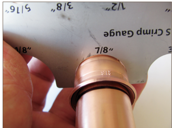
Figure 11.22. Correctly crimped fitting
