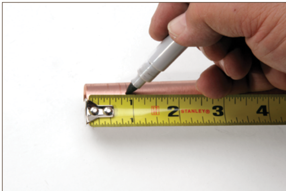
Figure 11.12. Measuring depth of insertion
