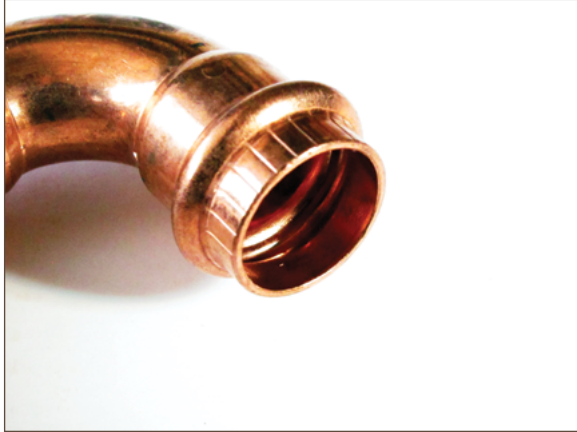
Figure 11.11. Press fitting (NOTE: Missing o-ring)
