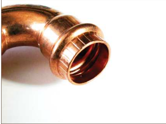
Figure 11.11. Press fitting (NOTE: Missing o-ring)
