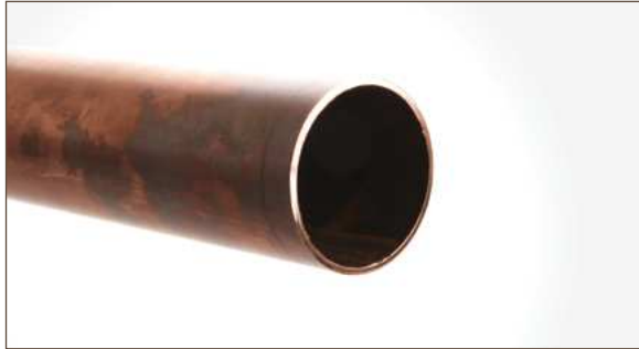
Figure 10.3. Square-cut tube end
