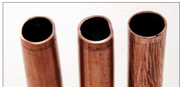
Figure 11.4. Inspect tube for imperfections
