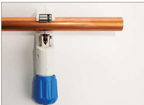
Figure 11.6. Cutting the tube square
