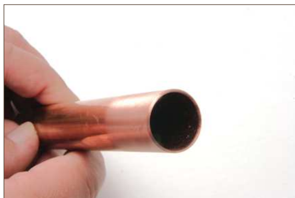
Figure 11.10. Properly prepare tube end
