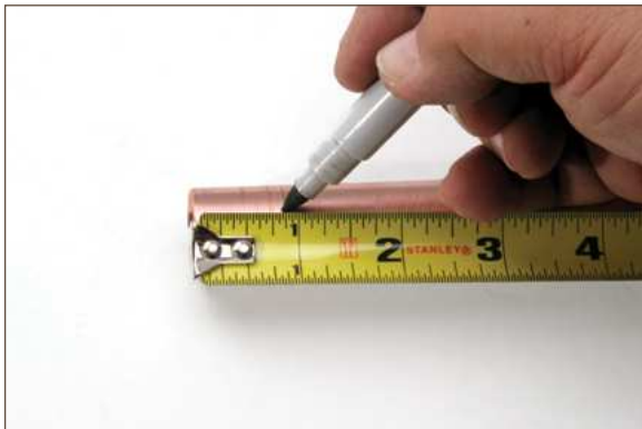
Figure 11.12. Measuring depth of insertion
