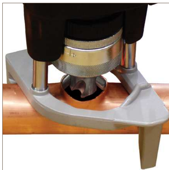
Figure 13.7. Forming the outlet
