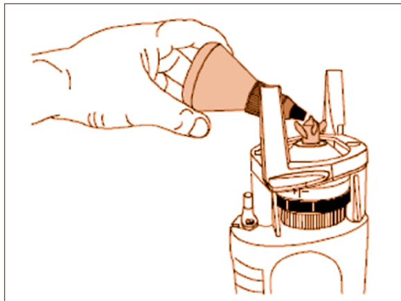
Figure 13.3: Lubricating the drill head
