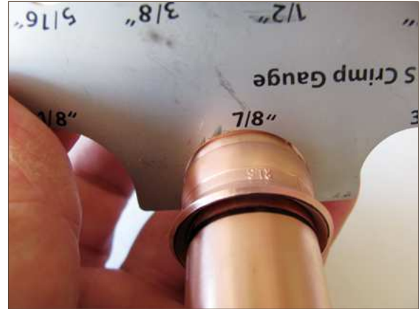
Figure 11.23. Correctly crimped fitting
