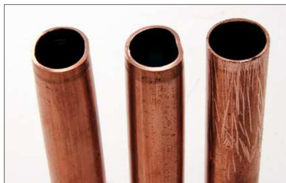
Figure 10.1. Inspect tube for imperfections
