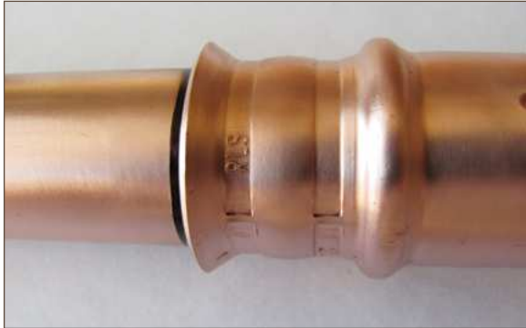
Figure 11.20. Press jaw crimp mark
