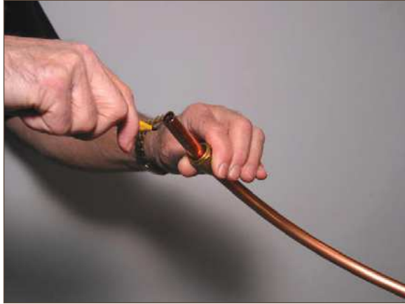
Figure 9.3. Reaming Prior to Flaring the Tube End
