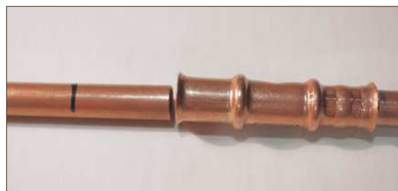
Figure 11.18. Tube marked for insertion into HVACR fitting
