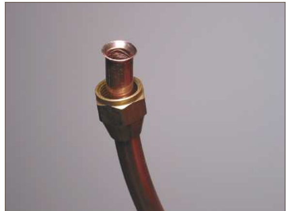
Figure 9.5. Completed Flared Tube End
