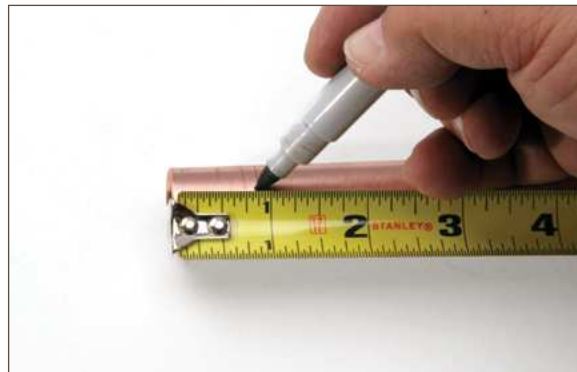
Figure 12.10. Making insertion depth
