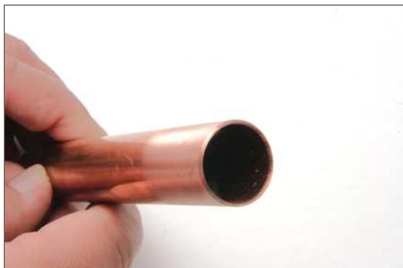
Figure 12.8. Chamfered tube end
