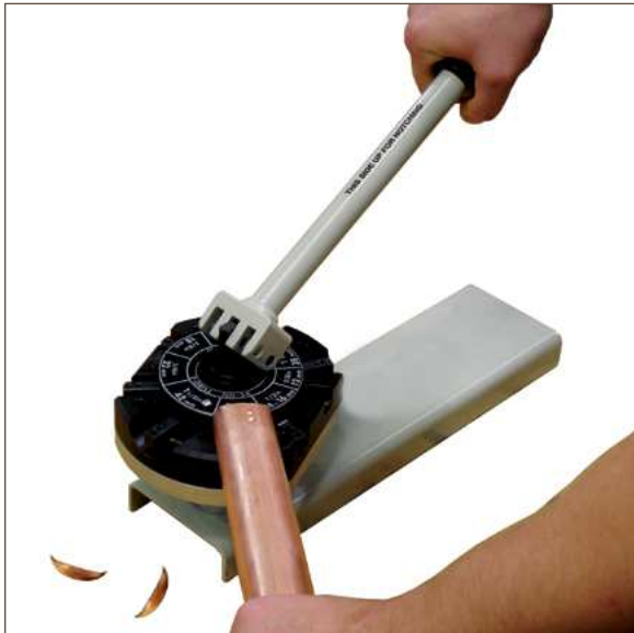
Figure 13.9. Using the notching and dimpling tool
