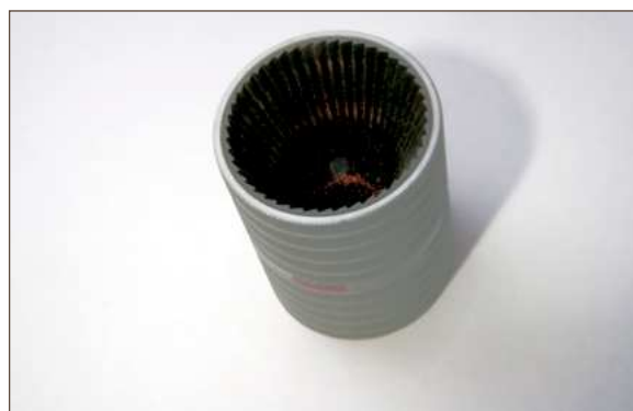
Figure 11.9. Combination tool for I.D. and burr removal
