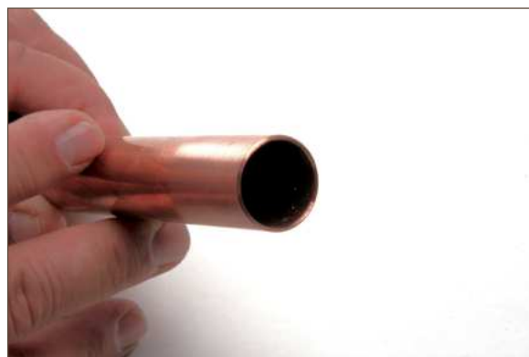
Figure 13.8. Reamed and deburred branch tube end
