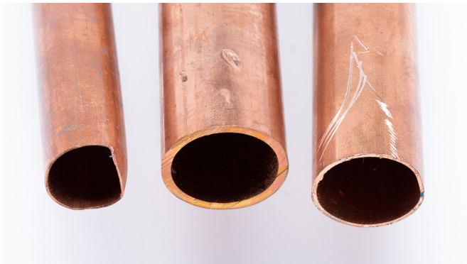
Examples of Damaged Pipe: dents, gouges and scrapes should be cut off to expose good pipe ends.
