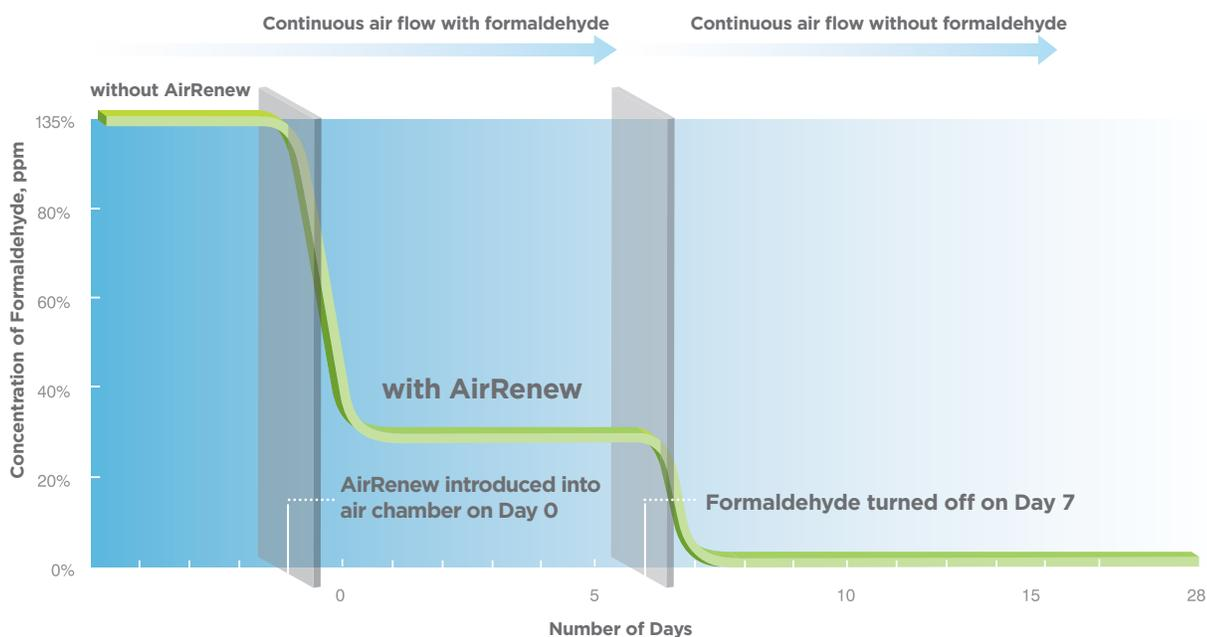
ISO 16000-23: Indoor air — Performance test for evaluating the reduction of formaldehyde concentrations by sorptive building materials. The effectiveness of the AirRenew process has been proven by tests conducted in accordance with ISO 16000-23, and validated by ULE through their Environmental Claims Validations program.
