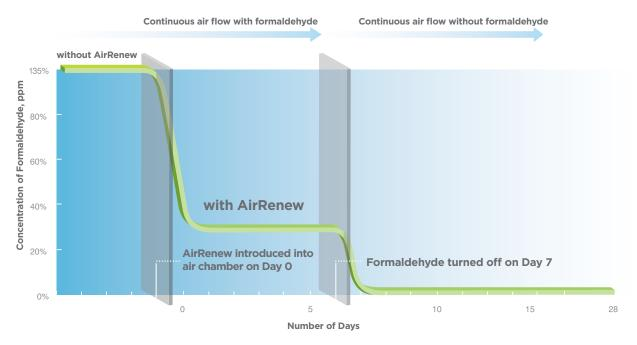
ISO 16000-23: Indoor air — Performance test for evaluating the reduction of formaldehyde concentrations by sorptive building materials. The effectiveness of the AirRenew process has been proven by tests conducted in accordance with ISO 16000-23, and validated by UL Environment through their Environmental Claims Validations program.
