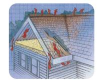
As a general rule, there should be one square foot of net open vent area for each 150 square feet of attic floor when there is no vapor retarder at the ceiling. If the ceiling has a vapor retarder, provide one square foot of net open vent area for each 300 square feet of attic floor area.
