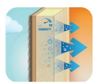
During the cooling season, when outdoor relative humidity is typically high, MemBrain changes its permeance to increase drying potential.
