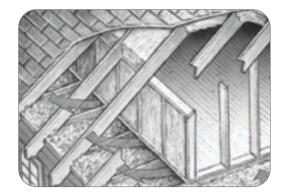
After creating access to each cavity, install baffles to allow ventilation air to flow from the eave vents (if present) up over the horizontal insulation in the floor of the cavity (see page 13). Also install baffles to allow the air to flow between the roof deck and the insulation in the sloped ceiling cavities (as described for cathedral ceilings on page 19).
