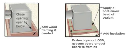
Seal chases where flues penetrate into attics with non-combustible materials. In addition, install dams to keep the insulation a safe distance away.
