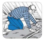
When using insulation batts, place them one after the other until you reach the center. Simply cut the insulation to fit. Install insulation the same way on the opposite side of the attic, working from eaves toward center.
