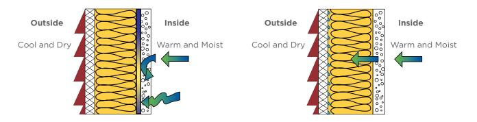
In warm, humid regions with a long air conditioning season and high exterior humidity, water vapor sometimes moves in a continuous flow from the warm exterior to the cooler interior of the home.
