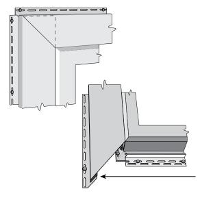
Snap the completed top lineal into the previously attached starter strip. Bend the rain tabs of the top lineal down into the receiving pocket of the side lineals.
