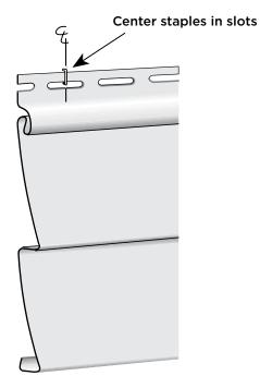
NOTE: Do not nail too tightly. To permit expansion and contraction, panels should hang freely from nails. This allows the panels to move as the temperature changes. Drive the nails until there is between 1/8" to 1/16" of space between the nail head and the nailing flange.
