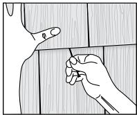
Push on the back button of the snap rivet to secure the clip to the panel. Repeat over each locking tab area.
