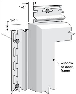
remaining vertical nails and all horizontal nails: place in center of slots
