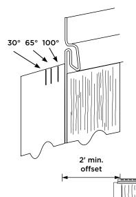
If the ambient temperature is less than 45°F, lap the panel to the first (30°) mark.
