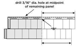
Install the next panel by positioning it below the starter strip and next to the first panel. <u>Push in and up</u> to lock the panel into the starter strip and the side tabs of the first panel. Space the second panel according to the panel temperature at the corresponding temperature indicator lines.
