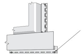
Snap the lineal in place and secure by nailing (or stapling) it through center of the nail slots.
