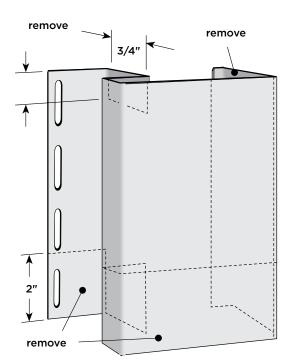
To create the header, first cut a  $7^{\prime\prime}$  piece of  $5^{\prime\prime}$  lineal. Measure and trim as shown.
