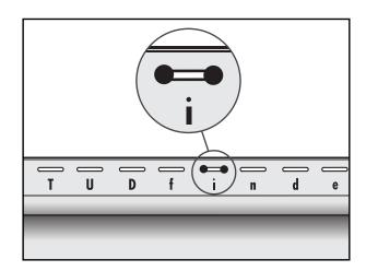
NOTE: Ensure that nail/staple penetration is at least 3/4" into a stud (1-1/4" into the stud olus sheathing) to comply with ASTM D4756 (specification for vinyl siding installation). Also be sure to allow 3/8" for expansion and contraction between panel ends and trim when install temperature is greater than 40° F, and 1/2" for expansion and contraction between panel ends and trim when install temperature is less than 40° F.
