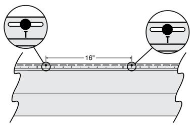
Standard 12' panels feature 10 nail slots every 16", with one of the 10 letters in the word "STUDfinder" centered directly under each slot. Locate the first stud and fasten the siding to it in the center of the nail slot. Notice which STUDfinder letter appears below the slot.
