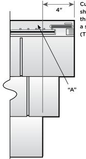
Cut off the top shingle and cut through to form a straight edge (T5 perfection)
