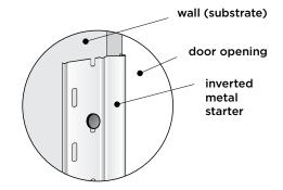
If the opening has no framework, such as a brick molding, use the metal starter in place of the Window and Door Starter Strip. The lineal's locking leg will fit behind the aluminum starter and into the receiving pocket of the Window and Door Starter.
