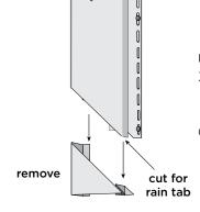
Use a triangle to create a 45° angle or measure 3-1/2" in from the locking leg.
