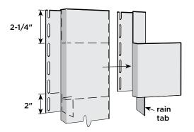
To create the header end cap, cut a 9-1/4" piece of 5" lineal and trim as shown.
