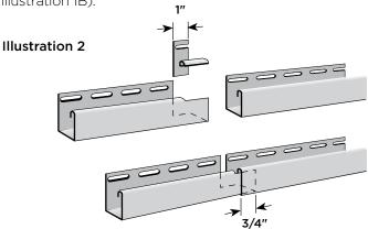
Install inverted J-Channel along the top of the wall, under the eave. Here again, leave a 1/4" gap between J-Channel and cornerposts. Overlap J-Channels 3/4" to allow for expansion. When positioning the upper J-Channel, be sure to allow for expansion of the siding panel. In most cases, position the J-Channel at a point equal to the length of the panel plus 5/8" (1/4" for upper expansion and 3/8" for lower expansion).
