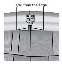
6. When you reach the top panel, use the cornerpost that was cut previously to create the starter course and cut this piece to length and nail it with a color matched finish nail. Measure from lowest butt edge of the last panel installed to the cornice receiver. Subtract 1/4" from measurement and cut your corner to that length. Leave 1/4" between the top corner piece and the cornice receiver.
