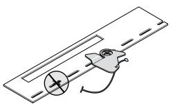
You must install the cam clip and the snap rivet at the same time. Installing the rivet before the clip may cause the rivet to mushroom and prevent it from keeping the cam clip securely in place.
