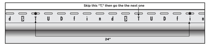
NOTE: Monogram XL 25' panels must be "center pinned" to control expansion and contraction. To do so, locate the center nailing slot of the panel and drive nails into both ends of the slot (see illustration). This is only done for one nail slot per panel.
