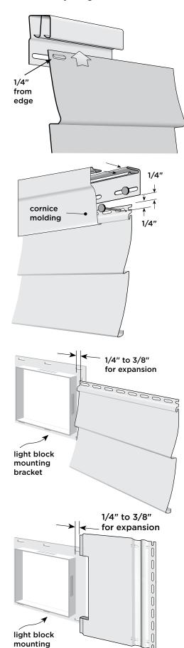
To install, lock the bottom of the cut panel into the panel below. Push the top edge into J-Channel or undersill trim. Tabs will catch in the trim and hold the panel firmly in place.
