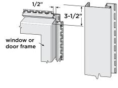
Measure the height of the window. Add 7" if using 3-1/2" lineals for the header and bottom lineal. (When using 5" lineals at header, add additional material). Cut lineal to length.
