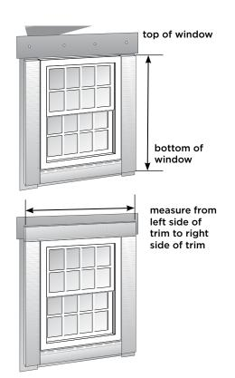
these pieces to the left and right sides of the window, verifying that the top edge of each section lines up with the top of the window and the bottom edge of each section lines up with the bottom edge of the first piece of trim already applied.
