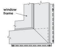
Snap the side lineals into place and secure using nails or staples.
