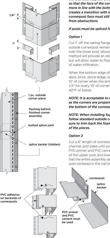
NOTE: If the transition material allows, the bottom 3/4" of the channels may be removed from the outside cornerpost so that the face of the corner may be positioned lower and more in line with the bottom of the siding. This method creates a transition with more pleasing aesthetics. The outside cornerpost face must still maintain 3/8" or 5/8" clearance from obstructions.
