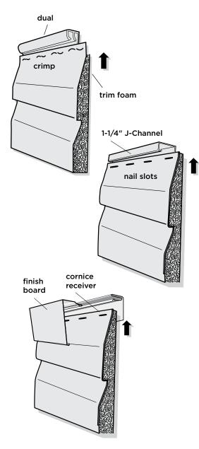
When installing CedarBoards XL 16'8" panels, the succeeding studs are at every 8th slot. When you apply the next panel, adjust the overlap, as necessary to line up with studs and repeat the steps above.
