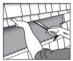
Pry the nails out of the nail hem of the damaged panel.
