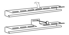
NOTE: If you don't have the proper receiver for the soffit, you can modify J-Channel to create an F-receiver. Simply cut slots in the nail flange area where the receiver will be nailed to the wall, bend back the flange, and nail the flange to the wall.
