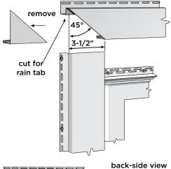
Use a triangle to create a 45° angle or measure 3-1/2" in from the locking leg.
