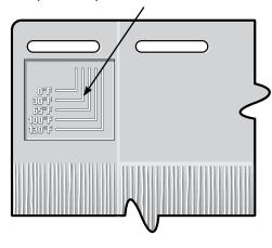
PRO TIP: When installing Cedar Impressions over foam insulation, extra care needs to be taken to verify that adequate space is left between all nail heads and the panel.
