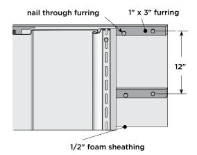
always position topmost nail in topmost full nail slot with vertical applications
