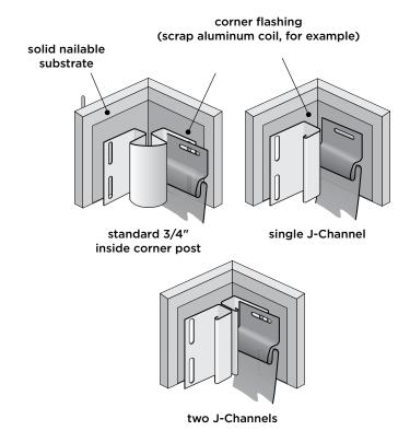
If you have to splice the inside cornerpost, cut 1" off all but the outer face of the lower post. Lap 3/4" of the upper post over the lower post, leaving 1/4" for expansion.
