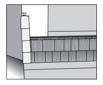
Angle the panel into the cornerpost and slide to the left until the side tabs clear. Next, slide the panel to the right until you have the correct temperature marks on the panel lined up.
