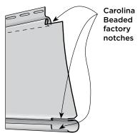
NOTE: Whenever you cut a panel to be used in an overlap area, you also have to duplicate the factory notch at both the top and bottom of the cut end.
