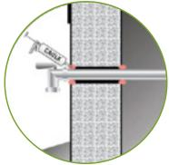
After gypsum board is installed on the interior, seal all gaps around windows, doors, outlet boxes and other penetrations.
