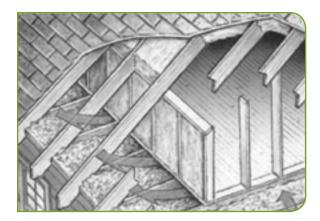
These attics can be a source of significant heat loss, so they should be thoroughly air sealed and insulated. The typical treatment is to insulate the walls and floors of these cavities.
