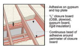
Another major area of air infiltration is the attic access opening. This may be a push-up hatch, a pull-down stair or a finished walk-up stairway. These areas should be thoroughly sealed and insulated. There are several insulated attic hatch cover designs that are excellent for this application.
