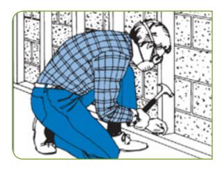
Place insulation between studs with the vapor retarder toward the interior of the home. Do not leave insulation exposed. Cover with an approved material such as gypsum board. Use only unfaced fiberglass insulation between wood framing and masonry chimneys. Do not place insulation in air spaces surrounding metal chimneys/flues or fireplaces.
