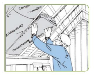
Working down the flange, staple about 8" apart until you reach the end of the batt. Do this until the batts reach the exterior walls. Fit batts tightly against each other.
