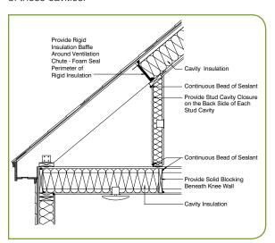
After creating access to each cavity, install baffles to allow ventilation air to flow from the eave vents (if present) up over the horizontal insulation in the floor of the cavity (see page 13). Also install baffles to allow the air to flow between the roof deck and the insulation in the sloped ceiling cavities (as described for cathedral ceilings on page 19).
