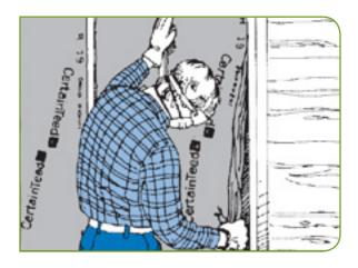
Fit the end of the batt snugly against the top piece of framing. Working down, staple the flanges, if attached, about 8" apart until you reach the bottom. Fit batts tightly against the framing bottom.
