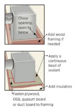
Seal chases where flues penetrate into attics with non-combustible materials. In addition, install dams to keep the insulation a safe distance away.
