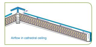
The insulation should be stapled or held in place by pressure against the sides of the rafters. An air space (at least 1") between the insulation and roof sheathing, ventilated at the ridge and soffit, is recommended.
