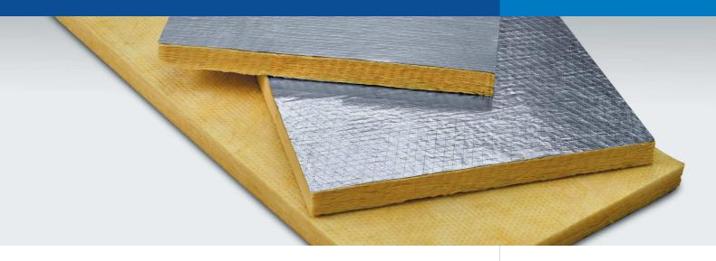
CertaPro Commercial Board is used where board stiffness properties are required. CertaPro Board is used in exterior curtain walls, interior walls and floor/ceiling assemblies, as an exterior insulation on HVAC ducts and plenums or in constructions where framing is not present, and also functions as an exterior insulation when covered with a weather barrier. It is also used as thermal insulation on tanks and vessels.
