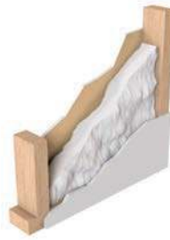
Figure 10: Conventional wood stud construction, single layer gypsum wallboard each side, 3-1/2" thick fiberglass insulation in wall cavity. STC: 34.
