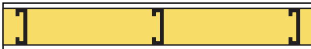
Rating: 1 hour non-bearing (U465 or W440) Single layer 5/8" CertainTeed Type X 3-5/8" steel studs on 24" centers 3-1/2" CertainTeed fiberglass insulation
