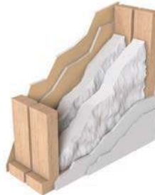
Figure 13: Double stud construction permits twice the thickness of fiberglass sound absorbing insulation. STC rating of 66-67 is excellent. See page 36.
