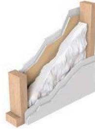
Figure 11: Conventional wood stud construction, double layer gypsum wallboard each side. Increased mass boosts STC rating to 55. See page 35.
