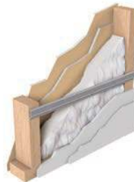
Figure 12: Resilient channels help minimize transmission of vibration through wall. STC rating of 57-59 considered acceptable for most uses. See page 35.
