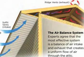
This system creates a condition in which the roof temperature is equalized from top to bottom, supplying a uniform air flow along the entire underside of the roof deck.
