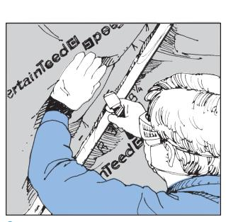
Working down the flange, staple about eight inches apart until you reach the end of the batt and do the same thing until the batts reach the top of the ceiling. Fit batts tightly against each other.
